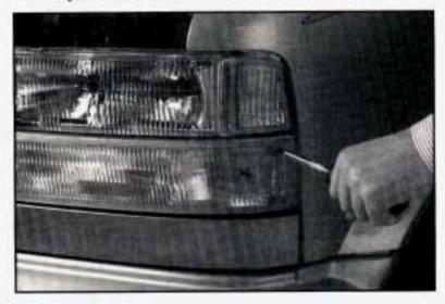
Remove the two screws from the side marker/turn signal lamp.
